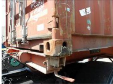
Figure 6.2 Mud in corner fitting
