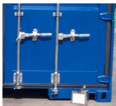
Figure 5.26 Handles on same side
