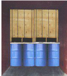
Figure 7.27 Mixed stow, dry over wet goods
