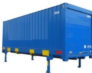
Figure 5.6 Swap body landed on support legs
