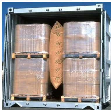
Figure 7.9 Gap filled with a central dunnage bag
