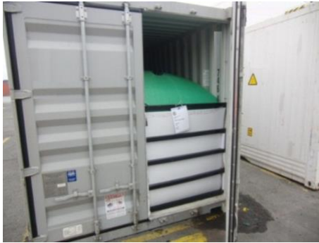
Figure 7.51 Container fitted with flexitank
