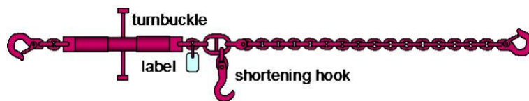
Figure 7.18 Standard chain lashing with shortening hook
