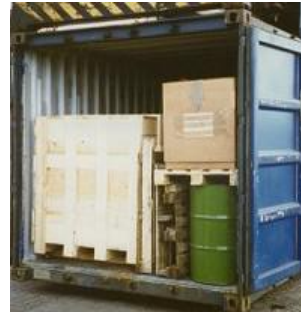
Figure 7.28 Mixed stow, use of pallets
