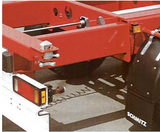
Figure 2.1 Twistlock on a road vehicle
