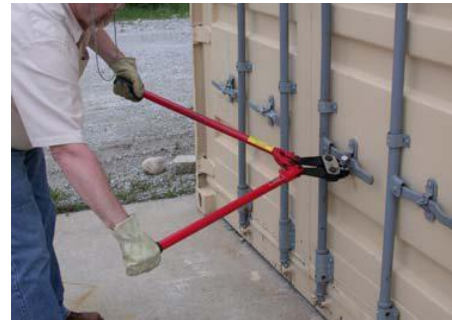
Figure 5.11 Cutting the seal
