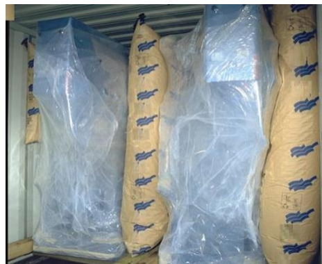
Figure 7.10 Irregular shaped packages blocked with dunnage bags
