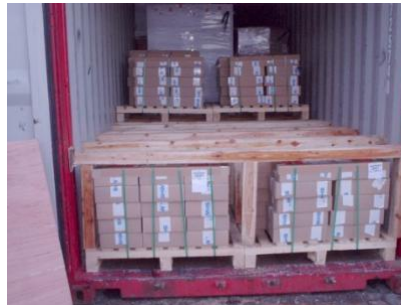
Figure 7.2 Timber temporary floor
