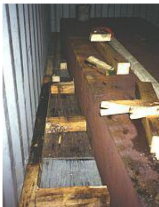
Figure 7.45 Transverse blocking of steel slab
