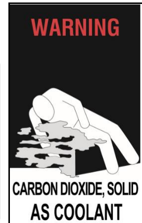
Figure 5.19 Dangerous atmosphere label
