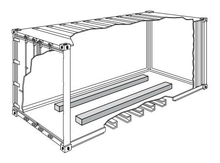
It is possible to extend the resting length of the cargo by using solid wooden or steel beams, but not more than 100 cm at each end of the load. It is important that the weight is distributed lengthwise on the container floor.
