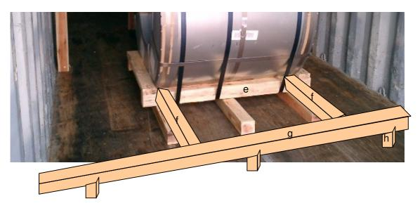
Both pieces (f) need to be placed between (e) and (g), all in the same height. Best to lay pieces (f) on the bedding and put the timber (g) on top of supports (h) with the same height as the bedding. Square timber (g) to be set with its ends into the corrugated side walls of the container.
