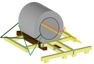
Finally the coil is to be secured by 4 nylon belts, each from each corner, like a closed circle.
