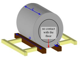
length should be 20cm longer (10cm each side) than length of the coil to place on this bedding on each end timber for blocking in length direction. Maximum free ends (b) have the same limits as written in Part A.
