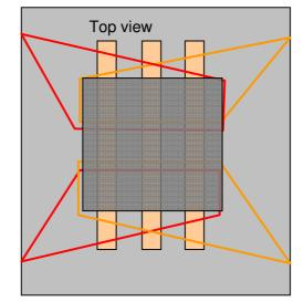
As the lashing eyes of a container can take only 1-2t, the strength of lashing material need not more than 2t.
