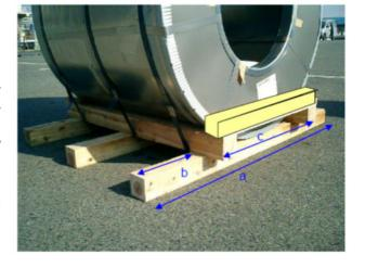
If not possible to meet these requirements, coils are too heavy for loading on timber bedding. Then steel bedding or other container types like flatracks required. Pls contact first your sales office, when you intend to ship heavier coils.
