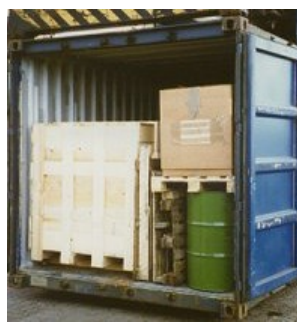
Figure 7.28 Mixed stow, use of pallets
