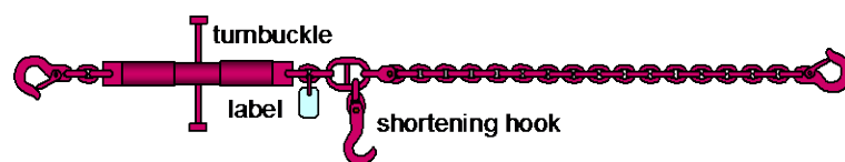
Figure 7.18 Standard chain lashing with shortening hook
