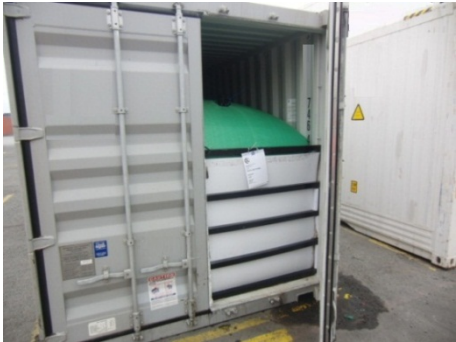
Figure 7.51 Container fitted with flexitank
