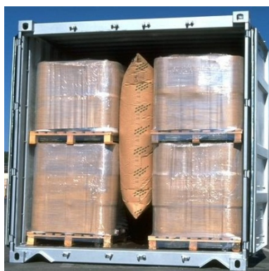
Figure 7.9 Gap filled with a central dunnage bag
