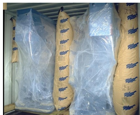
Figure 7.10 Irregular shaped packages blocked with dunnage bags
