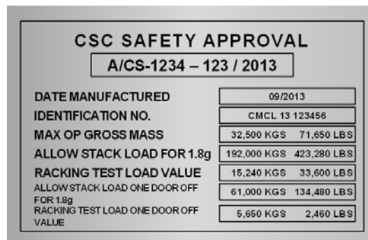
Figure 8.3 CSC safety approval plate for one door off operation
