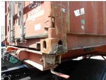
Figure 6.2 Mud in corner fitting
